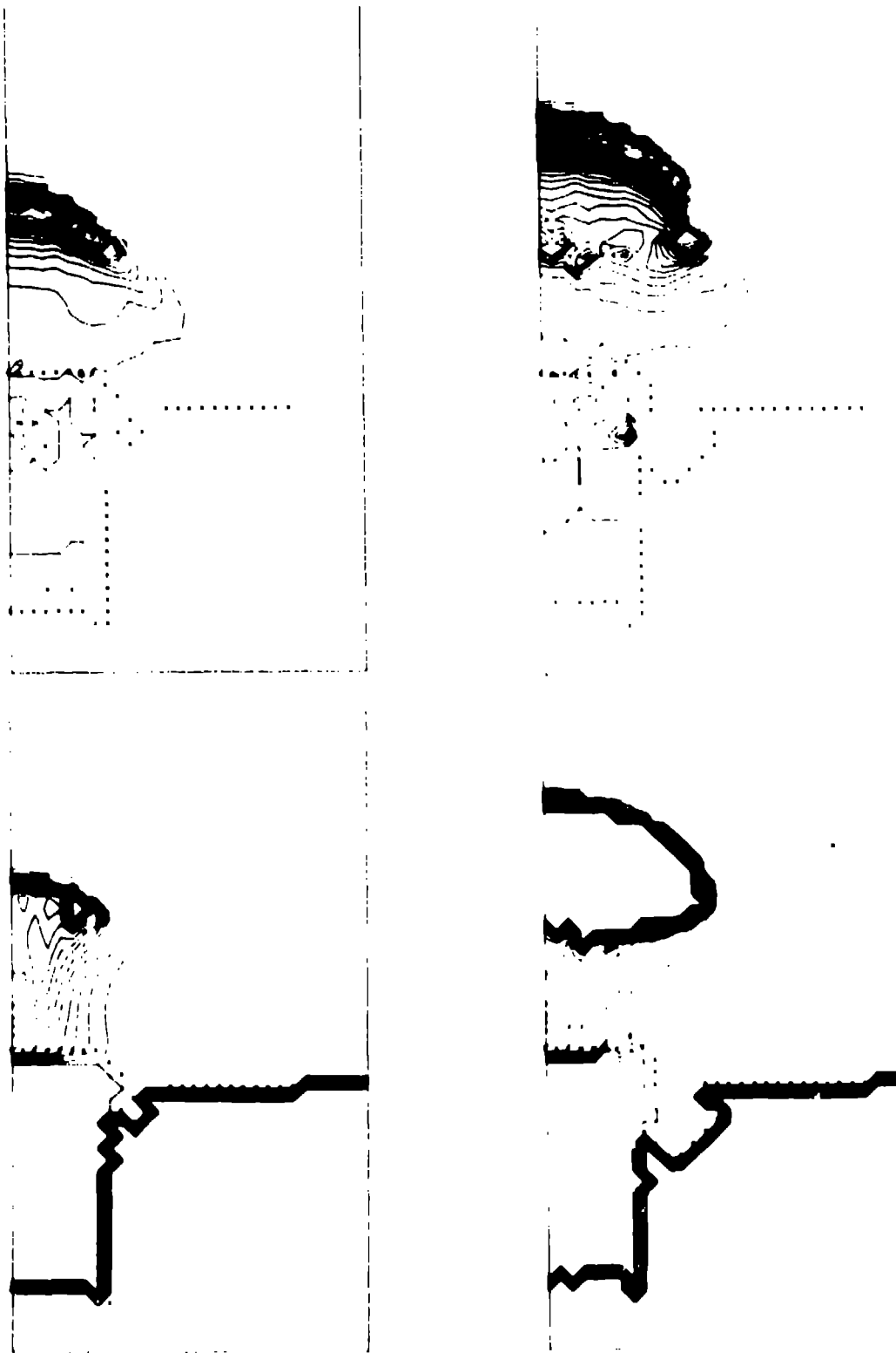
Figure 8. Isobars (Top) and Contours of Constant Mass Fraction at 1.91 \mu s (Left) and 2.38 \mu s After Impact by 7.62 mm (0.30 in.) Cylinder at 873 m/s (2864 ft/s)
